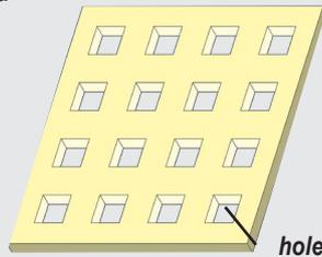
A three-dimensional “fishnet” structure was simulated. This consisted of a periodic array of rectangular subwavelength holes in a laminate consisting of magnesium oxide sandwiched between two gold layers.
