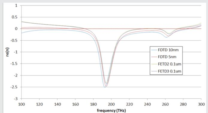
refractive index versus frequency for various FDTD and FETD resolutions: the negative index behaviour is shown below the red line
